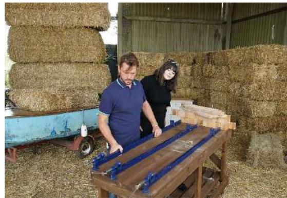
Once all strips have been cut line them all up on some sash clamps gluing them one by one with a waterproof PVA glue or Polyurethane glue.
