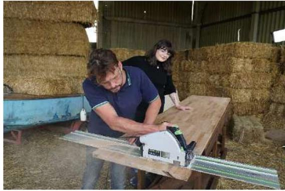
Use a circular saw to cut entire worktop into 75mm strips.
