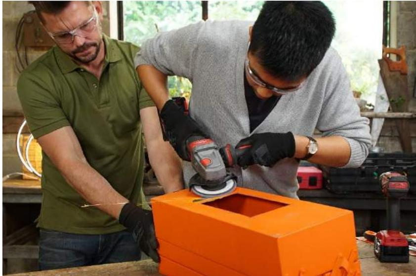
Grind away any paint where the flame may touch, this will prevent the paint from burning.
