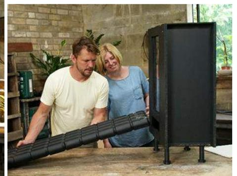
With the cabinet painted black to absorb all the sun's heat and the tubes inserted, place it in strong sunshine. The sun doesn't get hot enough in northern climes to dry food in the open air, as can be done closer to the equator. So this is a brilliant way of dehydrating food safely.
