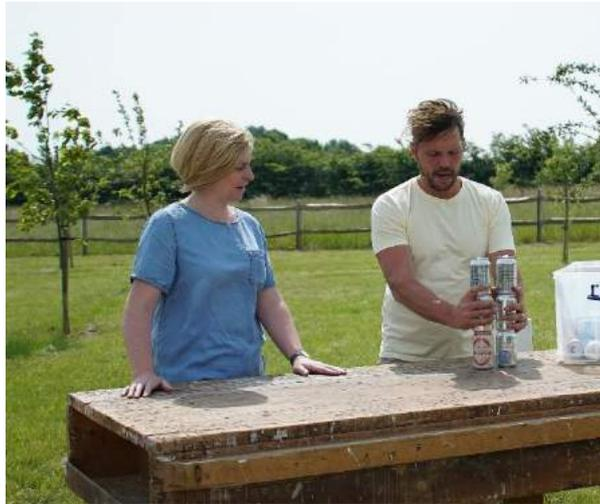
The cans are formed into tubes, using the mastic to fix them end to end and each tube to others. The sun will heat the air that is held within them. The set of cans will be tilted, so that the warm air rises through them and enters the cabinet. Holes in the base of each can lets the air move and painting them black increases the effectiveness of the solar heating.
