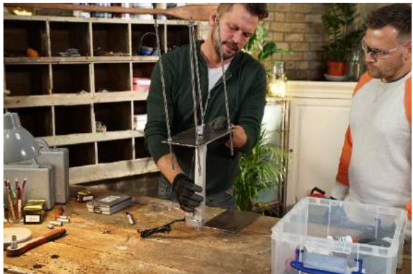
The frame is made to fit snugly inside the freezer with the actuator coming out the top.
