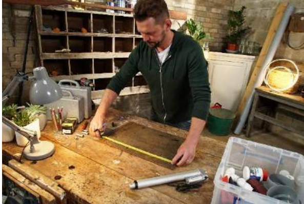
The frame is made to fit snugly inside the freezer with the actuator coming out the top.
